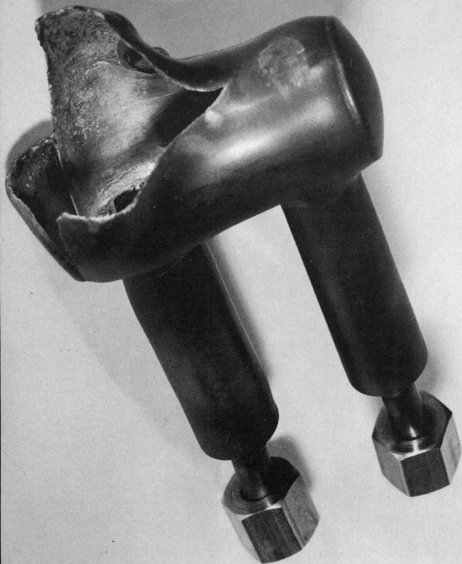
Figure 7 This nickel can, about 4 inches long and 1\frac{3}{4} inches wide (photo is approximately actual size), was ruptured by detonation of 100 milligrams of \text{XeO}_3 .
