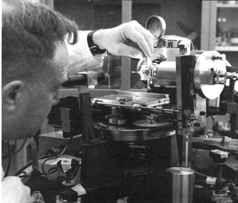
Figure 9 Argonne scientist Stanley Siegel positions a capillary containing \text{XeF}_4 in an X-ray camera. The capillary is the needle-like object in the center of the picture.
